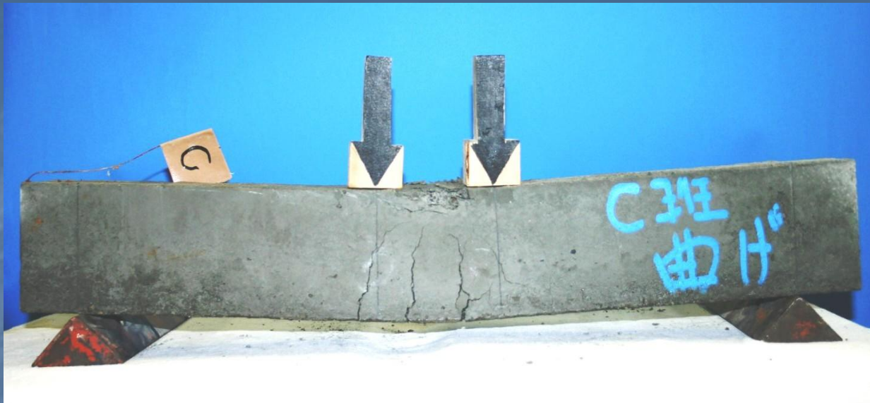
曲げ破壊 flexural failure
